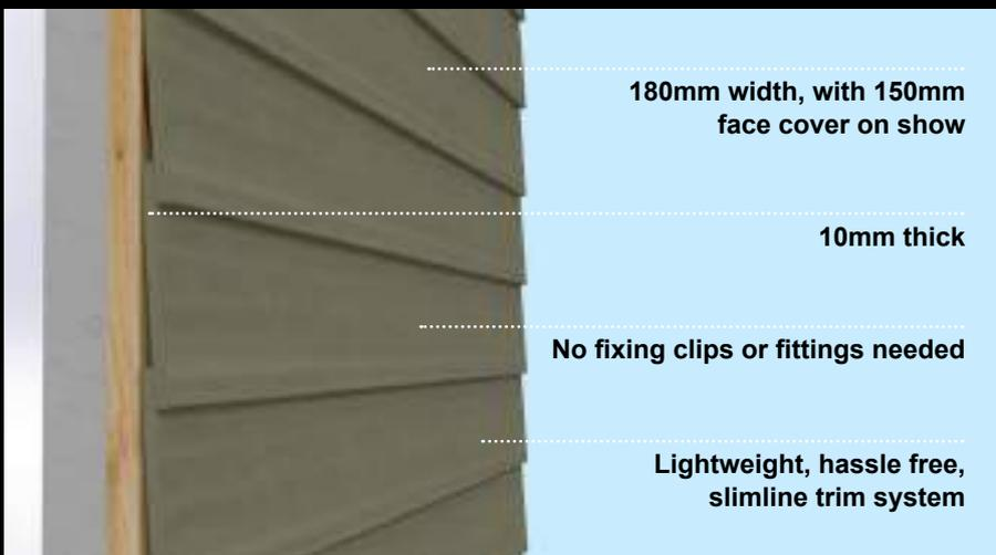
The 3660mm length cladding planks have a 180mm profile with a 150mm face and are designed to be installed in a "Weatherboard" style which overlaps at the horizontal joints to encourage water run-off for contemporary styling.
