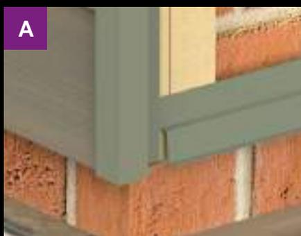
**Starter Trim:** Used to start a cladding run with a lip to cover the first batten. The Starter Trim will position the first plank at the appropriate angle for the remaining planks to be fitted, giving a uniform 'Weatherboard' finish.
