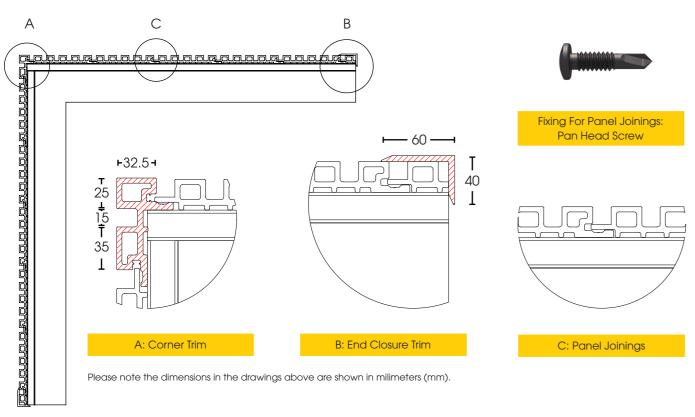
Pan Head screws should be used to affix the Dura Wall Panels. The screw should be positioned in the centre of the slotted hole to allow for expansion & contraction. Do not over tighten the screws and adjust torque settings according to your drill manufacturer's instructions. If the hole centres miss the battens, appropriate slotted holes must be drilled to allow for expansion and contraction.
